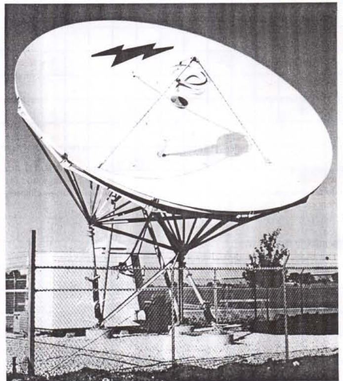
Figure 13.9 Shaped 10-m earth station dual-reflector antenna (courtesy Andrew Corp.).
